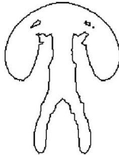
Fig. 20. The interface of merged bubbles on a cut plane at t = 0.22 .
