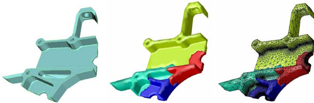
Figure 4.3: Hierarchy of domain decomposition: geometry model, partition model, and distributed mesh on 4 processors
