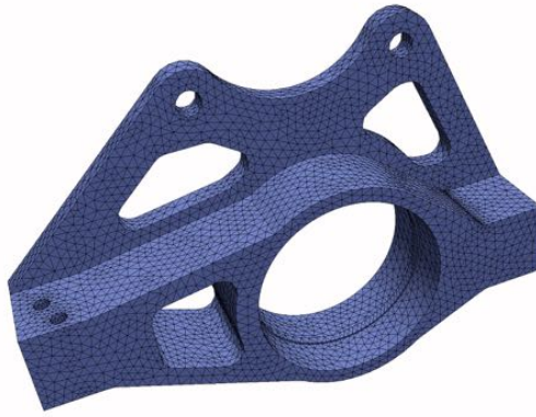
Fig. 2.2. Coarse mesh of the 2014 RPI Formula Hybrid suspension upright.
