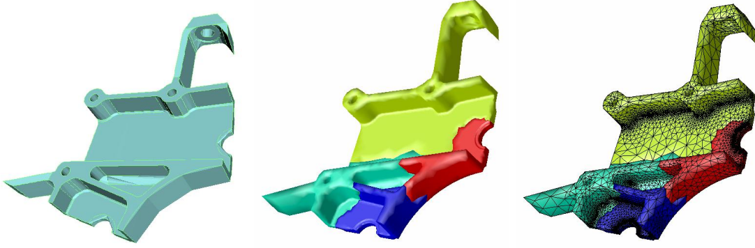
Figure 17: Hierarchy of domain decomposition: (left to right) geometry model, partition model, and distributed mesh on 4 processes
