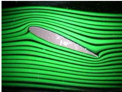
(a) A flow pattern around an airfoil [21]
