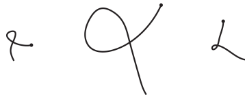
Fig. 6: An example of alpha gesture recognition. The program is able to recognize the inaccurate alpha gestures correctly though they are in different sizes and drawing directions.
